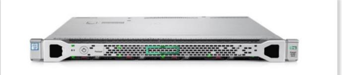
Runs on generic enterprise grade server hardware. Minimum hardware specification: Intel Xeon E5-2400 Family, 4 core processor - or better, 12GB RAM. Operating System - Microsoft Server 2022, or Debian GNU/Linux.
